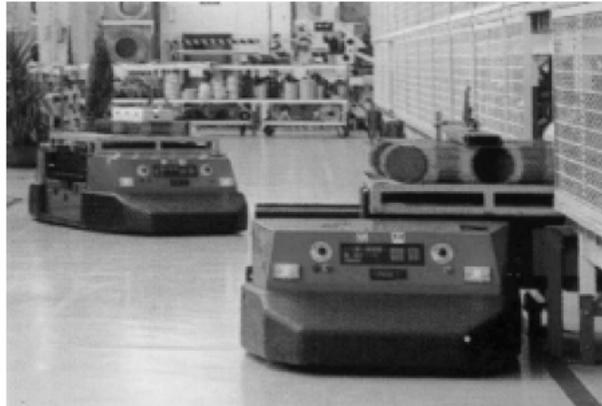
**Figure 1** AGV controlled by floor-imbedded guidance wire
