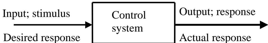
Figure 2.1: Simplified description of a control system (Nise, Norman [15])
