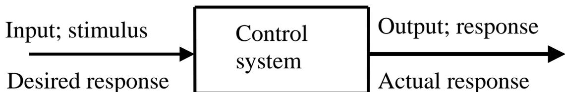
**Figure 3.1: Simplified description of a control system**
