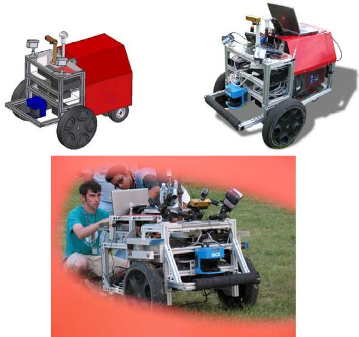
Figure 8 Bearcat Cub intelligent vehicle designed for IGVC
