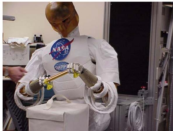
Figure 7. Robonaut, a humanoid robot from NASA
