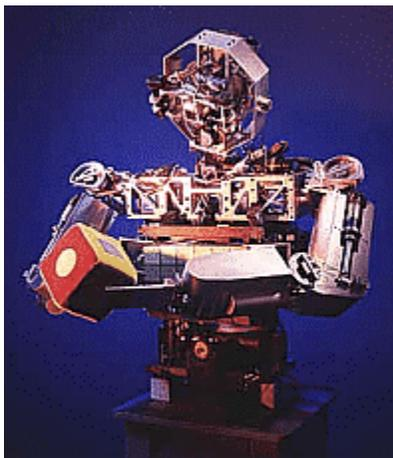
Figure 1. MIT humanoid robot, Cog, has twenty-two degrees of freedom
