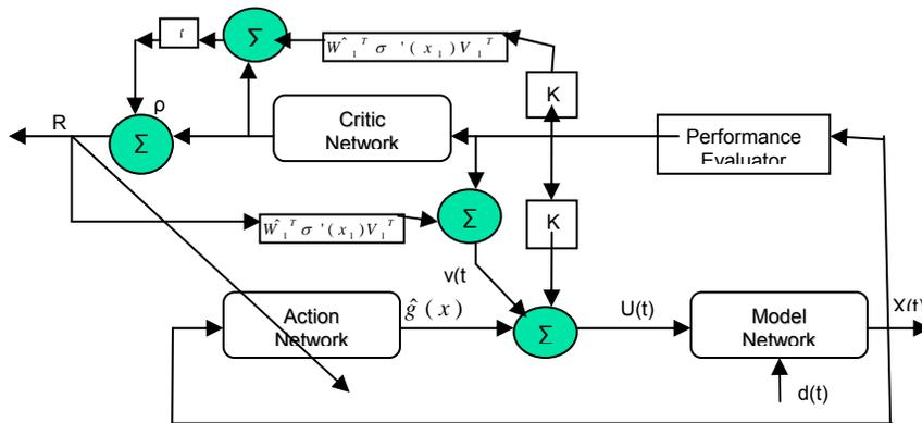
Figure 9. Adaptive critic learning structure<sup>35</sup>
