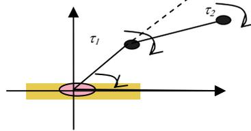
Figure 8. Two-link robot arm manipulator
