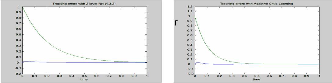
Figure 11 (a) Tracking error with 2-layer neural network vs. (b) Tracking error with adaptive critic learning (t=1sec)
