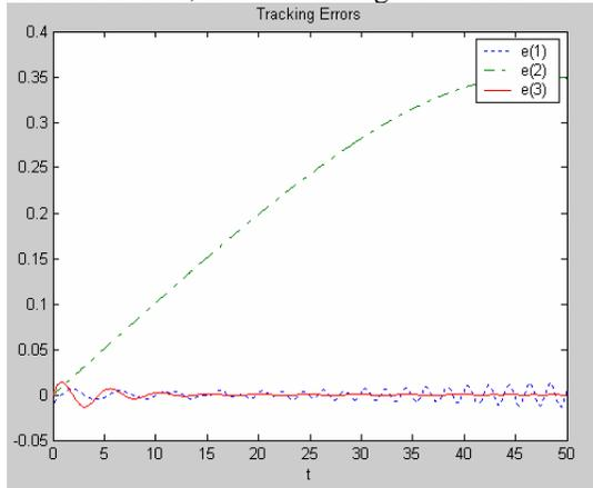
Figure 1: PID CT controller tracking errors versus time<sup>4</sup>.
