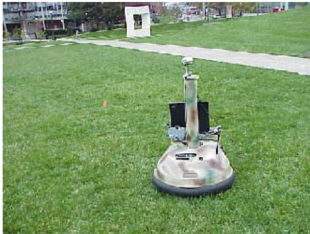
*Figure 5. Soil Sampling robot in a typical field test*
