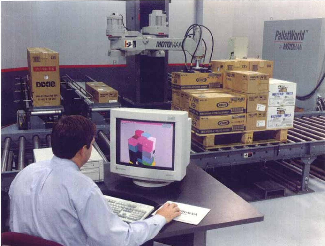
**Figure 3. Motoman mixed size/content palletizing workcell.**
