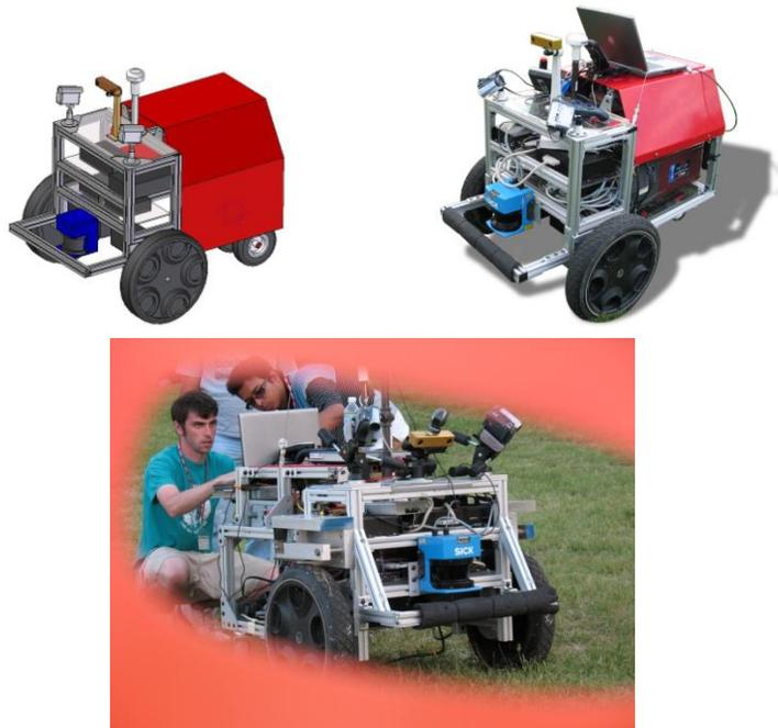
Figure 9 Bearcat Cub intelligent vehicle designed for IGVC
