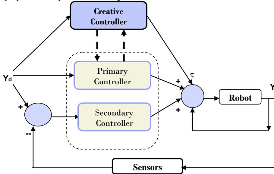
Figure 5 Block diagram of creative controller
