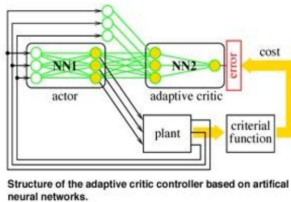
Figure 2 Structure of the adaptive critic controller <sup>8</sup>
