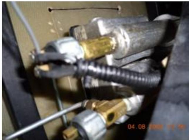
Figure 6. Hydraulic control cylinders
