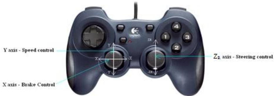
Figure 14. Joystick and the three control axes (<http://www.logitech.com/repository/95/jpg/450.1.0.jpg>)
