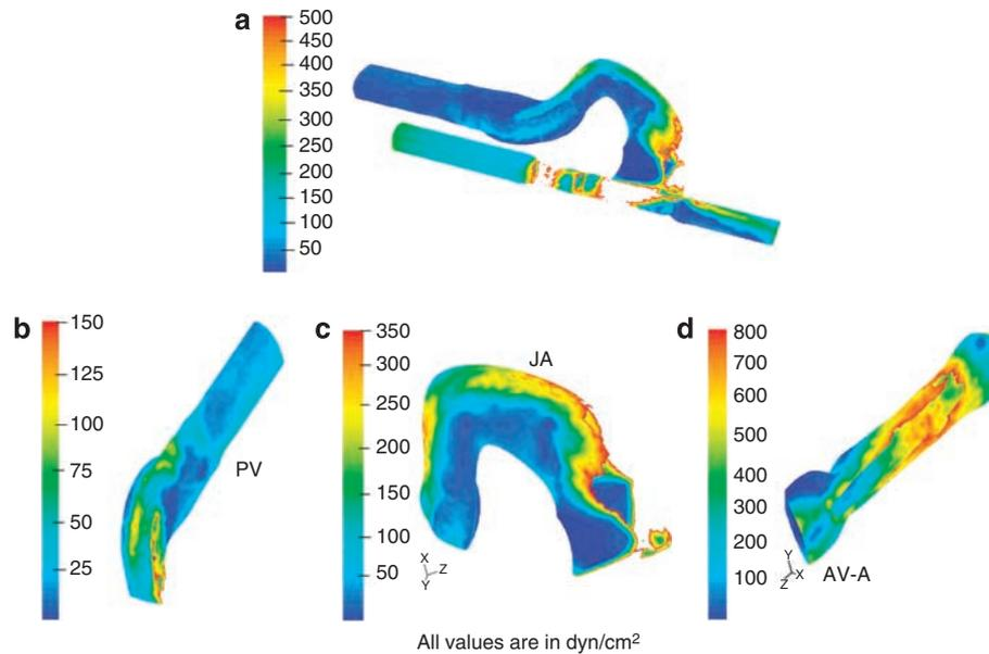
**Figure 4 | Wall shear stress contours of curved AV fistula configuration during peak flow.** (a) The WSS contours in the overall curved configuration. (b–d) The WSS contours in the different anatomical regions: PV, JA, and AV anastomosis, respectively.
