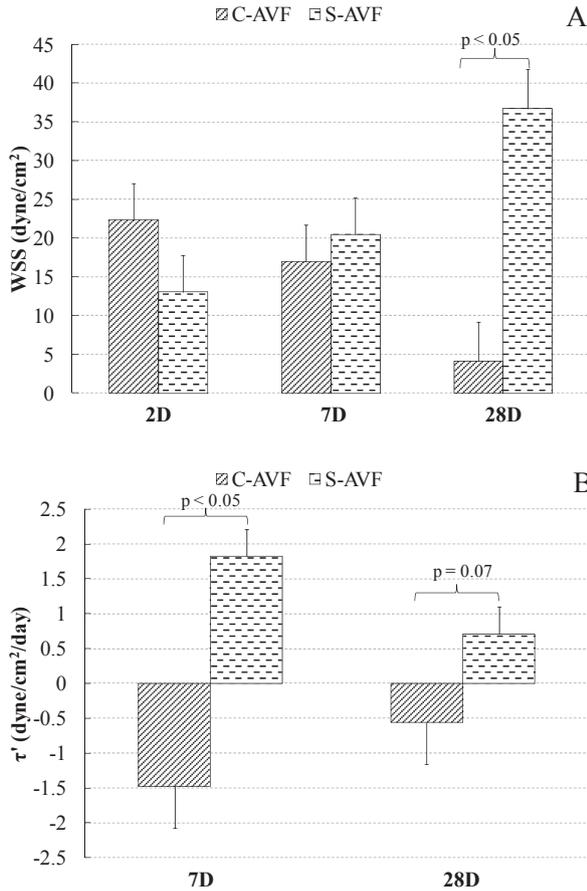
FIG. 7. (A) Variation in WSS levels and (B) temporal gradient of WSS over time for C-AVF and S-AVF.
