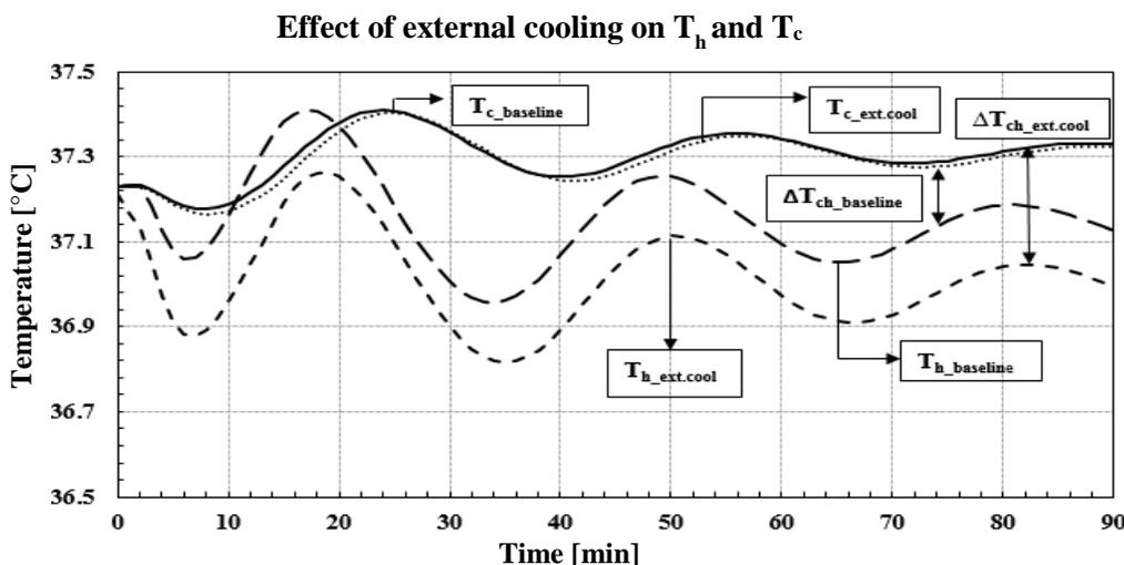
**Figure 1.** Computed  $T_c$  and  $T_h$  for the human body model during exercise a) without external cooling i.e. baseline b) with external head cooling of 232.8 W/m<sup>2</sup>.
