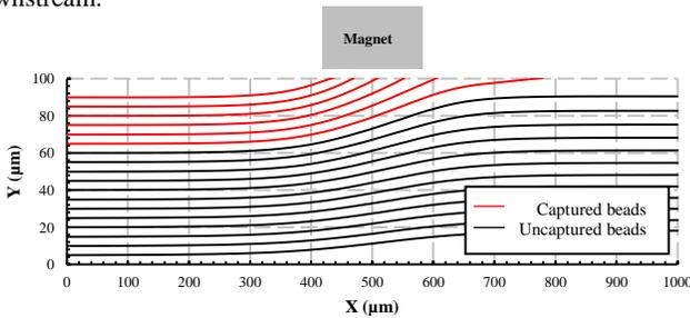
**Figure 2: Trajectories of the beads at  $E=250$  V/cm,  $M = 40000$  A/m**
