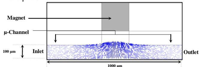
**Figure 1: 2D model of microchannel with magnetic field vectors**
