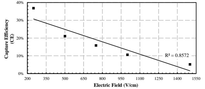
**Figure 3: CE at different electric fields,  $M = 40000$  A/m**
