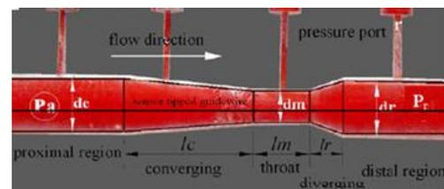
**Figure 1:** Test section of a 64% area stenosis
