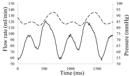
**Figure 2:** An example of flow and pressure pulse obtained.
