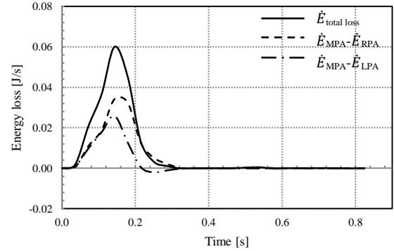
**Figure 3. Energy loss between the MPA and the branch PAs over the cardiac cycle.**
