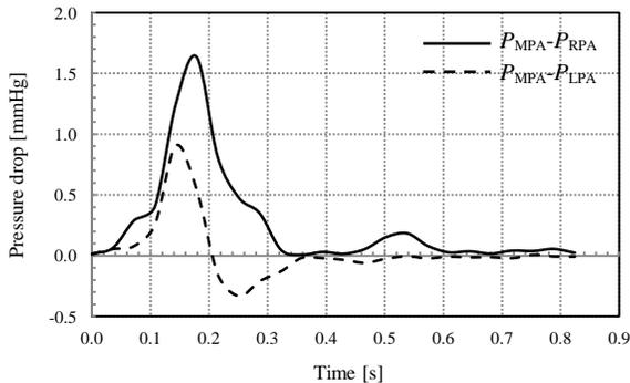
**Figure 2. The pressure drop between main PA (MPA) and the branch PA, RPA and LPA over the cardiac cycle.**
