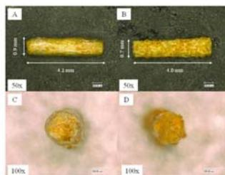
Figure 1. A. Top View of Coated Implant A; B. Top View of Uncoated Implant B; C. Cross section of coated Implant A showing PLA coating on the edge; D. Cross section of uncoated implant B.
