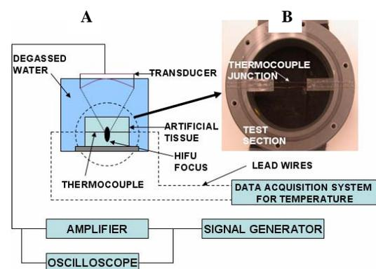
Figure 1A: Schematic diagram of HIFU apparatus
