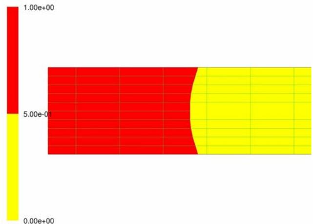
**Figure 1. Simulation mesh showing water in microchannel at t = 0.0581 seconds.**
