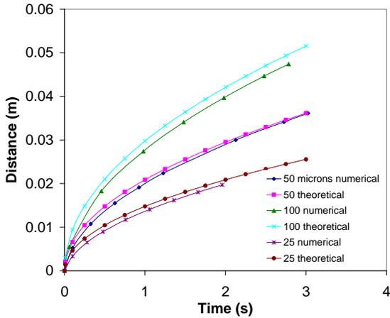
**Figure 2. Simulation results for water in 25, 50, and 100  $\mu\text{m}$  channels.**
