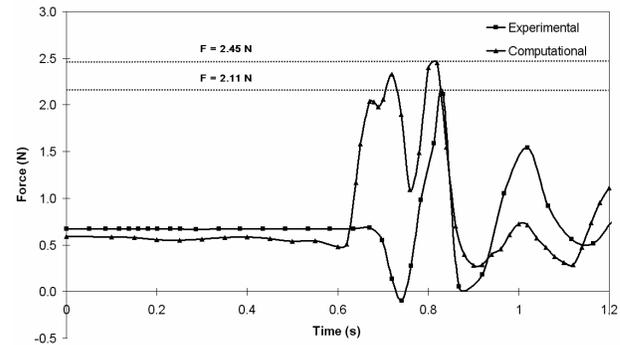
**Figure 4. Comparison of Experimental and Computational Drag Force.**
