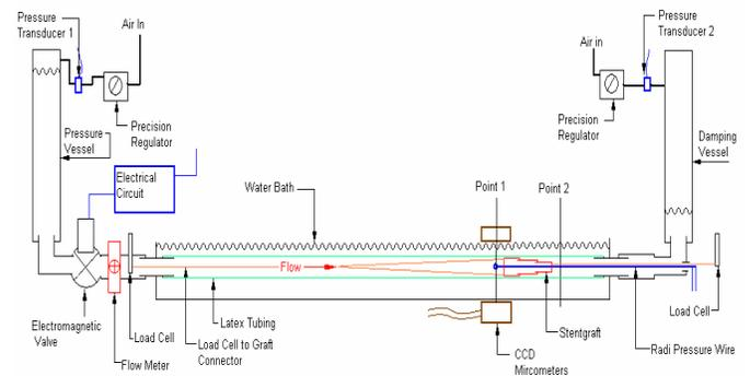
**Figure 1. *In-vitro* experimental set up**
