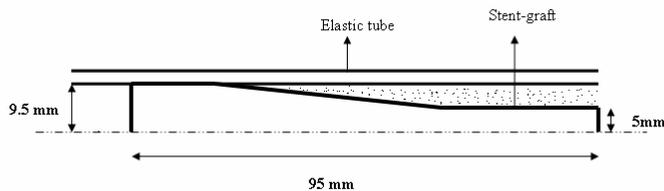
**Figure 2. An axi-symmetric model of stentgraft along with elastic tube.**
