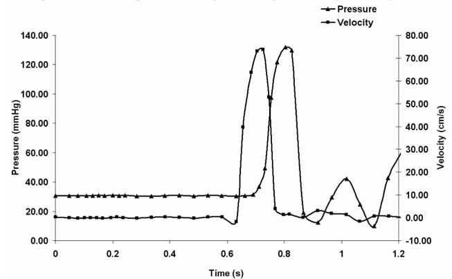
**Figure 3. Pressure and Velocity profile from the *in-vitro* model**
