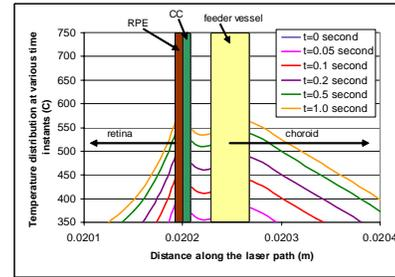
Figure 3b. Dye-enhanced absorption in the feeder vessel,  $Q=0.5 \text{ W}$ , spot 50  $\mu\text{m}$  dia. Tissue layer between feeder vessel and CC is 25  $\mu\text{m}$ .
