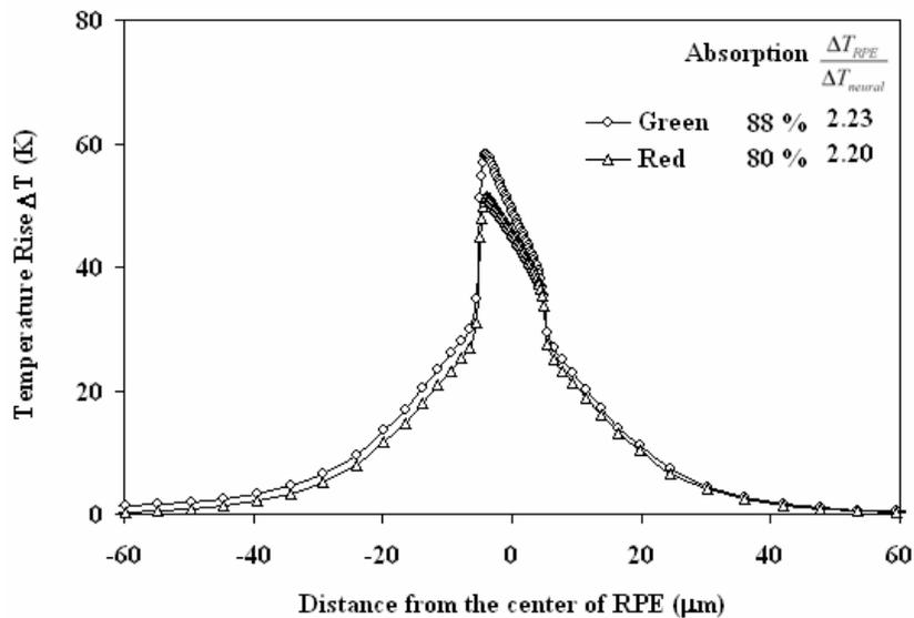
Figure 5: Temperature rise for different wavelength for 2 $\mu$ s pulsed laser at 5000 Hz
