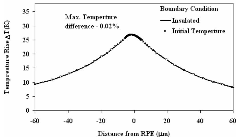
Figure 2: Validation of boundary condition
