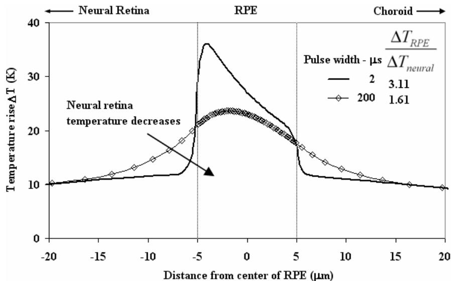
Figure 7: Temperature rise for 2 and 200 μs pulses at 1000 Hz after 100 number of exposures
