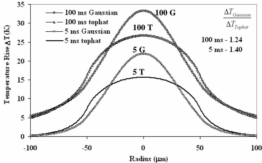
Figure 6: Comparison of temperature profile for Gaussian and top hat profile
