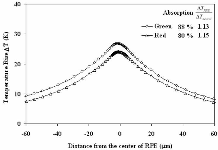
Figure 4: Temperature rise for different wavelengths for CW laser
