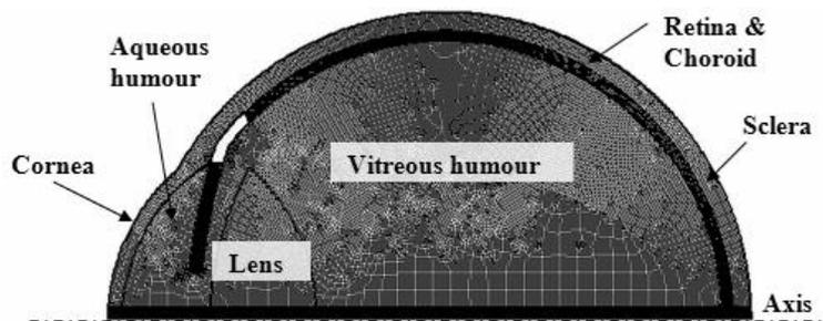
Figure 1. Two dimensional axi-symmetric model
