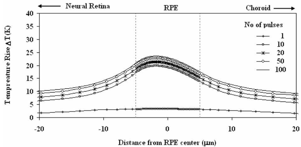
Figure 8b: Temperature rise for 200  $\mu\text{s}$  pulses
