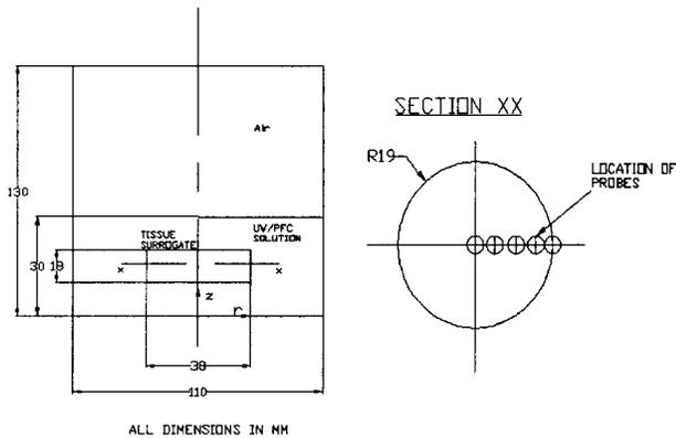
Figure 1: Experimental Setup for Simple Storage in UW/PFC solution.
