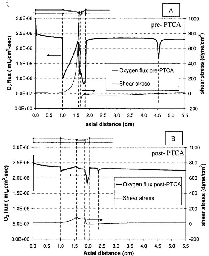
Fig 1: Comparison of O<sub>2</sub> flux to the wall and wall shear stress along axial length between pre- (a) and post- (b) PTCA stenosis.
