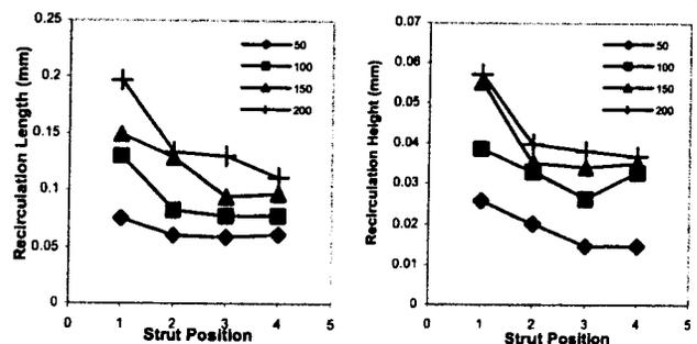
Figure 4: Variation of recirculation length and height near each strut for basal to hyperemic flows at  $t = 1.85 \text{ s}$
