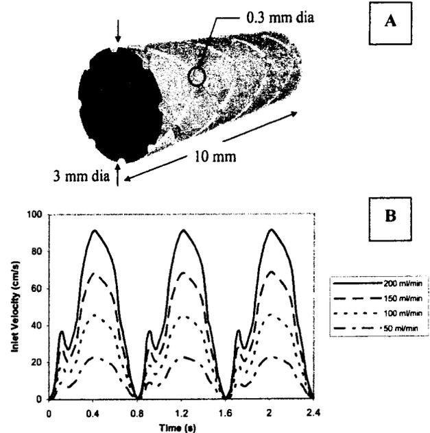
**Figure 1: Mesh plot of coronary artery with deployed stent (A). 3 consecutive pulse cycles for basal to hyperemic flows (B).**
