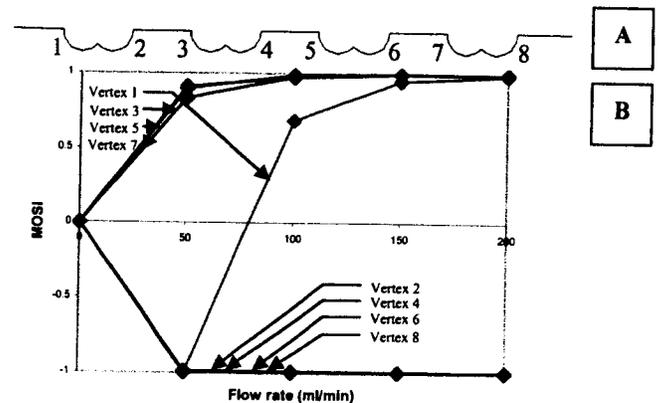
Figure 3: Schematic diagram of the locations of vertices 1 to 8 (Fig. A) and Variation of modified oscillatory shear index at vertices with flow rate (Fig. B)
