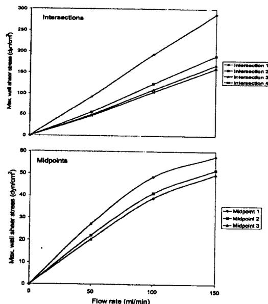
Figure 3: Variation of maximum wall shear stress with flow rate at strut intersections 1 through 4 of the stent and mid-point of the void locations 1 through 3 (shown in Fig. 1A).
