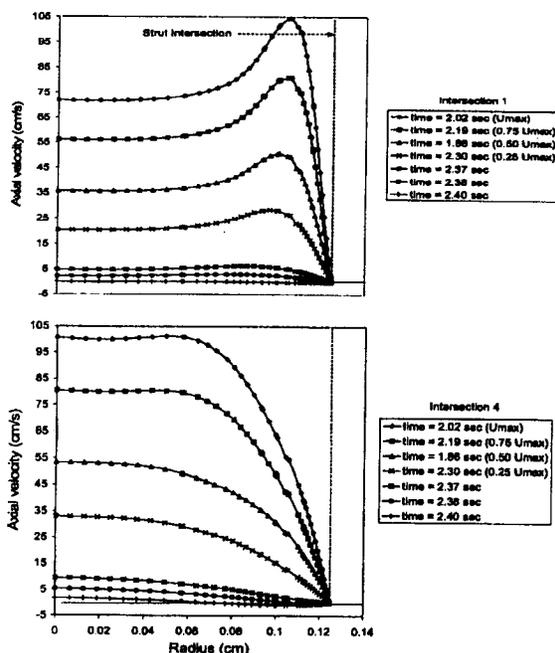
Figure 2: Axial velocity profile for near hyperemic flow of 150 ml/min at the entrance region (strut intersections 1 and 4 are shown in Fig. 1A) of the stent.
